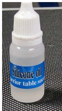
Wipe rods down with cloth or napkin then add 1 or 2 drops of silicone
