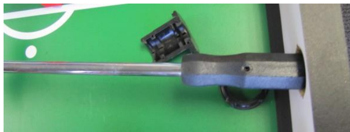
11. Guide handle through opening in near wall in proper position. Pull all the way in to allow other end of rod to clear far wall.
